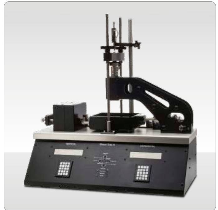
Standard Fully-Automated Rock Shear System
