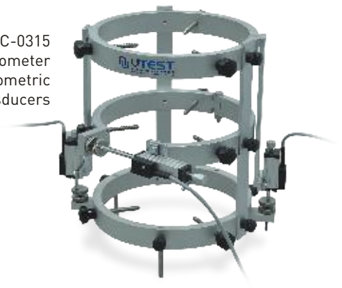
UTC-5507 Auxiliary Testing Frame for The Measurement of Deflection
