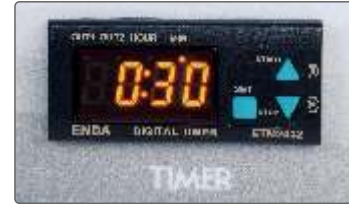
Sand Equivalent Shaker Timer
