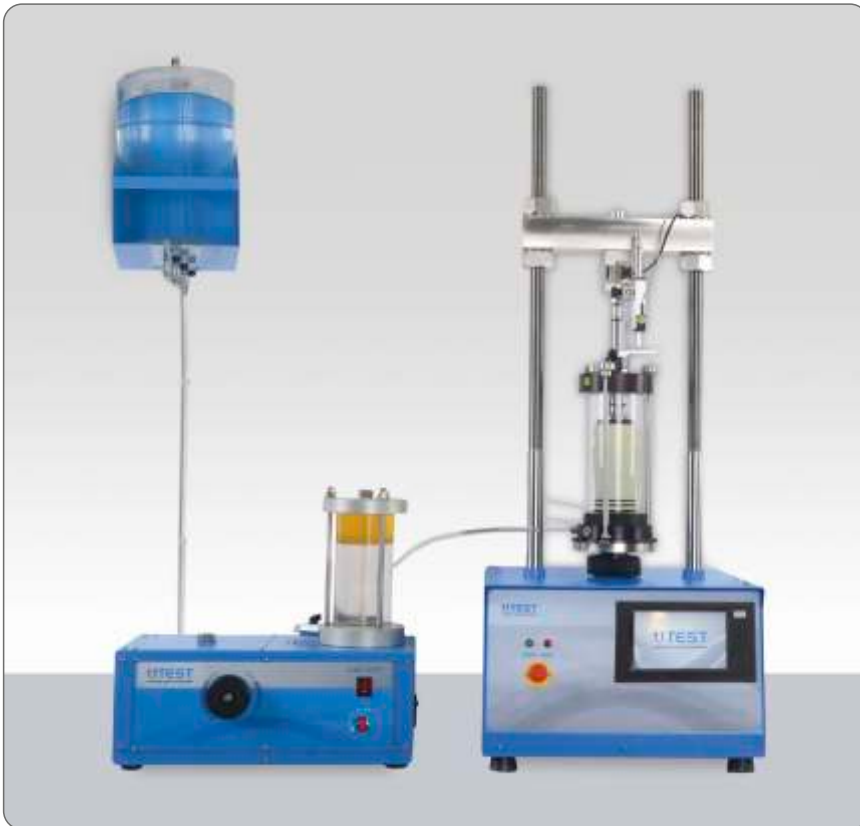
UU Only Triaxial Test Configuration
