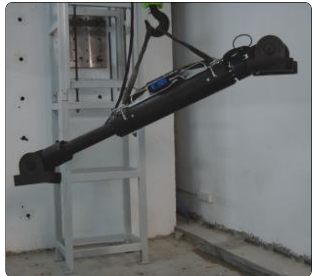
Long Travel, Fatigue Rated, 300 kN
