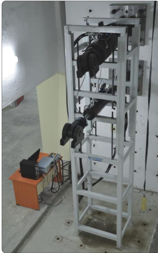
Actuators Mounted on Strong Wall
