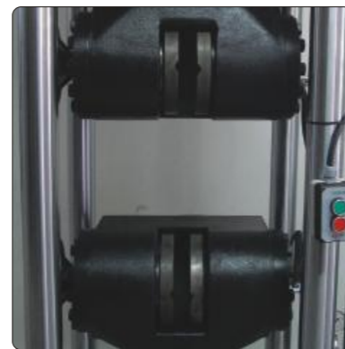
test space for tension tests
