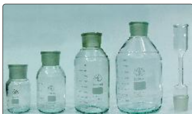
Pyknometers (Bottle Type) with Double Edged and Capillary Tubed Funnel
